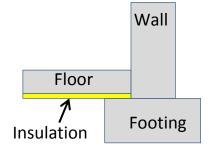
The barrier that the ants had to breach was a 2 foot wide by 18 inches deep concrete **Footing** that was laid around the perimeter of the house. A 11 inch thick continuous concrete **Wall** was poured on
